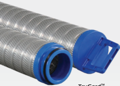
TruGard™ Cartridge Model EZ-PSFG Available in polyester or polypropylene media and micron ratings of 0.5, 1, 5, 10, 20 and 50.
